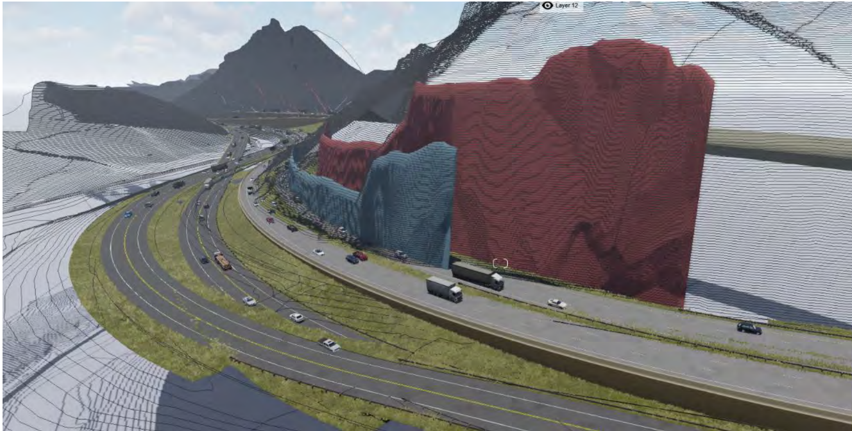
Figure A-3. Visual Simulation of Rock Cut on the north side of I-70 at MP 244, Tunnel Alternative, North and South Frontage Road Design Options*
