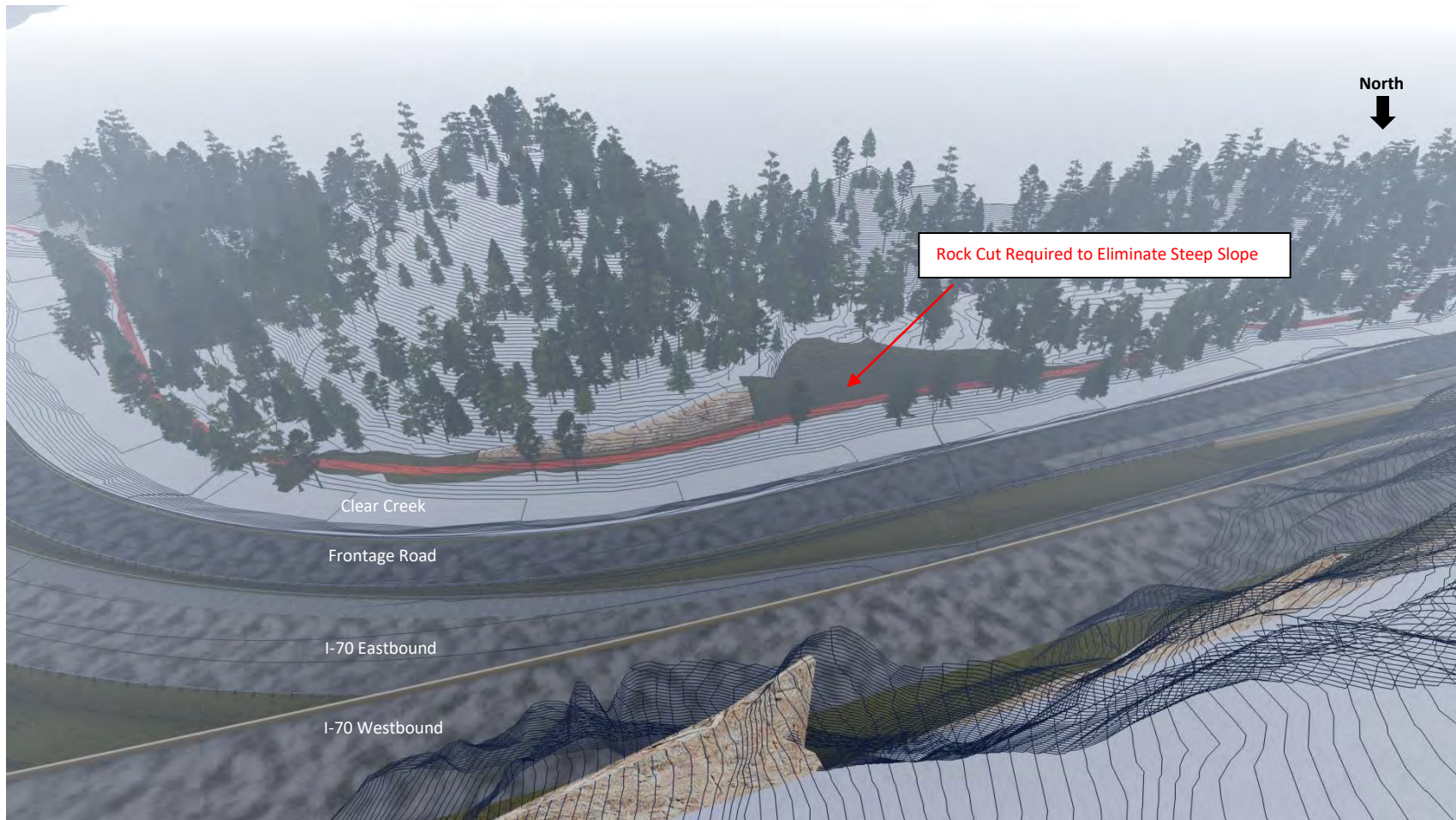
Figure A-1. Proposed Rock cuts for ADA Slope Compliance, Scott Lancaster Memorial Trail, Tunnel Alternative, North Frontage Road Option
